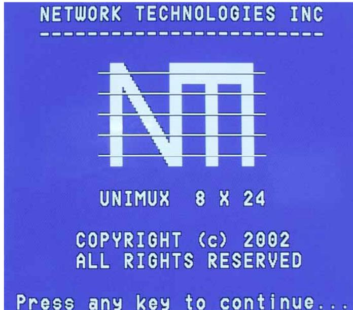
All the downstream switches should be powered ON before pressing any key. If there are USB extenders connected, they should also be powered ON. An extra time of about 5 seconds after powering-ON the last unit may be needed to complete the USB enumeration process. If the switch is a standalone unit (no downstream switches connected), the key could be pressed immediately.
