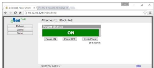
To control the power, click on the appropriate button. During power cycling, the Power Status bar will indicate the temporary status, with a blue background. Once the cycle is complete, the status bar will revert to its original condition.
