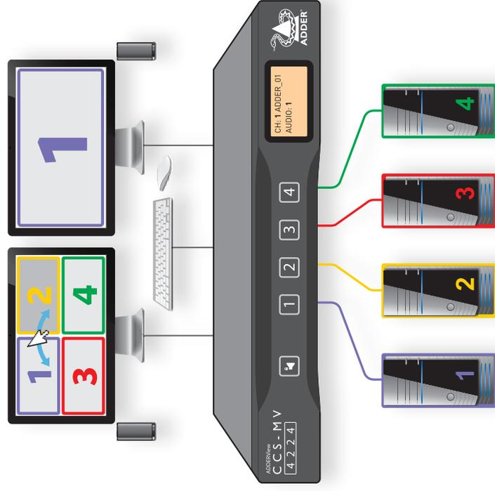
Switching between computers can also be controlled from the smart front panel or by using keyboard shortcuts or remote control/API.
