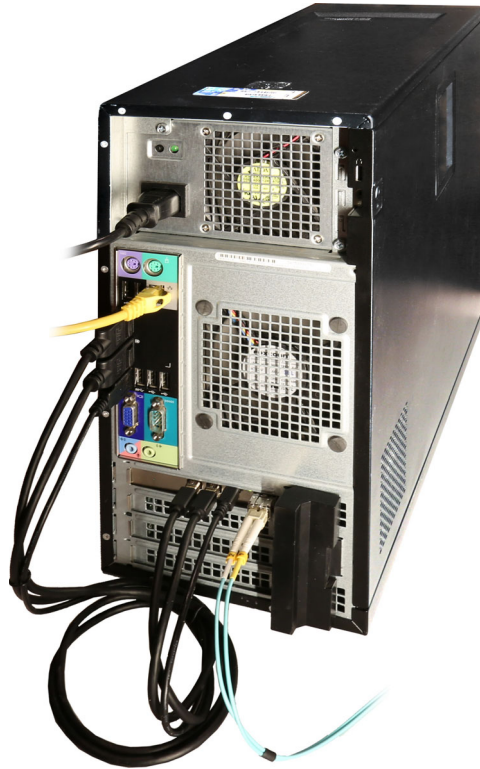
Figure 21. PCIe 2-port transmitter card with fiber
