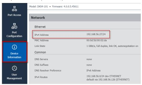
• To change network settings, such as setting a static IP address: Choose Device Settings > Network.
