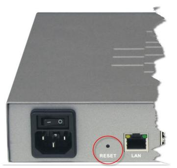
4. Continue holding the Reset button for 10 seconds. Once the device has been reset, two short beeps signal that the reset is complete.
