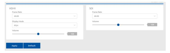
These 2 blocks are used to control the output modes, framerate and volume. For the HDMI model both outputs are HDMI, this is the SDI model's output.
