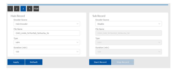
The record page allows user to change the video format that recorded to USB3.0 disk drive. On the top 1/2/3/4/PGM is the channel that desired to record; and the 2 block in the middle is the main/sub record format.
