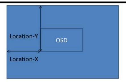
**Location-X**: OSD offset of X axis **Location-Y**: OSD offset of Y axis
