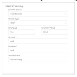
**Encoder Source**: User can select between main encoder and sub encoder.
