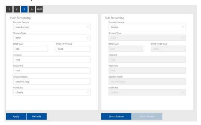
This page contains the GSM 400 streaming settings; user can decide which encoder's stream will send out and select streaming type here.
