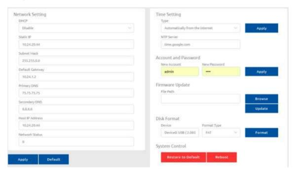
In the system page, user can set account /password, system reboot, format attached USB disk, check network status/setting and **Firmware Update** here.
