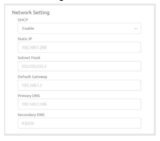
**DHCP**: Enable/disable DHCP feature. When you disable DHCP, please provide necessary network parameters.
