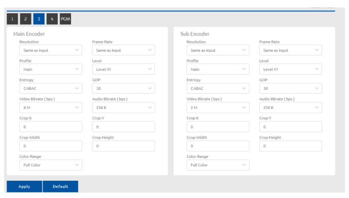
Encoder page contains **Main Encoder** and **Sub Encoder** 2 parts, which allows user to change video and audio encode, this page also provides user to change sub streaming encoder.
