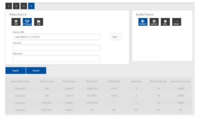
This page contains **input signal status**, input **Video Source** and **Audio Source** selection. Users can change input video property, source and check input video information here. User can select on the top 1/2/3/4 icons to change the channel that willing to adjust.
