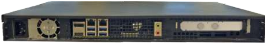
Model 8000-S1, Model 8000-S2 (Single SDI and Dual SDI input) On 8000-S1 the second BNC is a loop out
