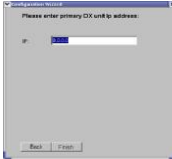
Figure 21 Primary DX unit IP address box
