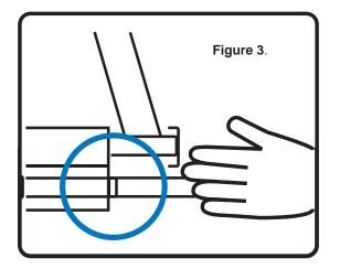
Push the LCD console drawer into the rack. (shown in Figure 3).
