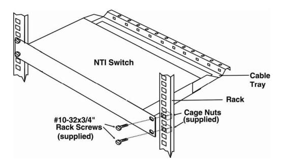
Figure 1- Secure switch to a rack
