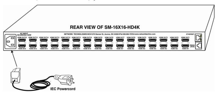
Figure 6- Attach AC power cord to VEEMUX
