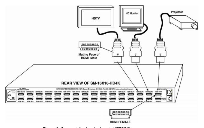
Figure 3- Connect display devices to VEEMUX
