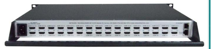
Rear View of SM-16X16-HD4K with cable tray installed
