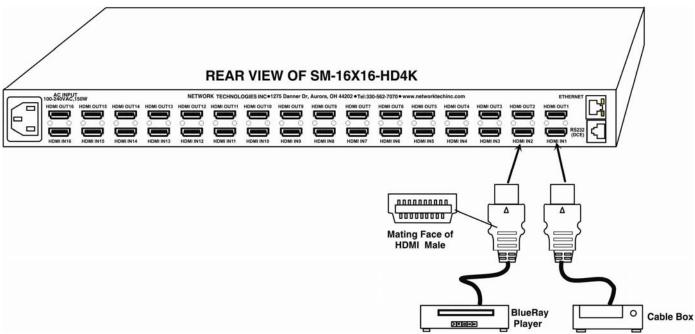
Figure 2- Connect video sources to VEEMUX
