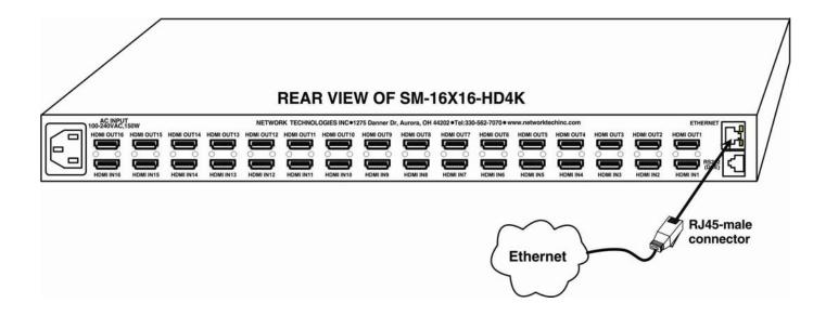
Figure 5- Connect VEEMUX to local area network
