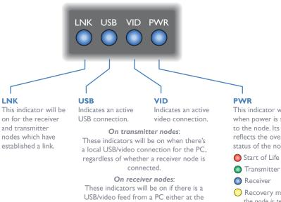
connected transmitter node or at the local feed through port (i.e. channel 0) of the receiver node.
