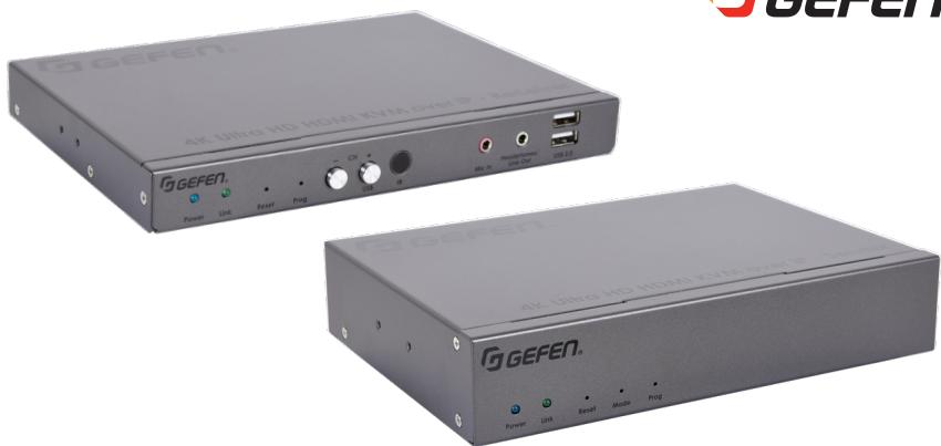
The Receiver's integrated USB hub with two USB 2.0 and two USB 1.1 ports accommodates touch panels, keyboard and mouse, and a variety of supported devices. This feature, along with analog audio inputs and outputs, make these products perfect to use in collaborative and interactive installations. To ensure maximum versatility and compatibility, the audio outputs on the Receiver units are compatible with both headphones and line level devices such as powered speakers.
