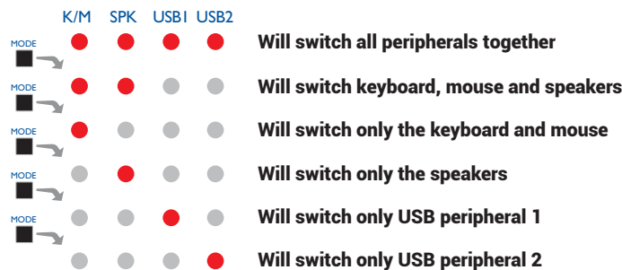
Figure 5-2. Changing the switching mode using the MODE button.
