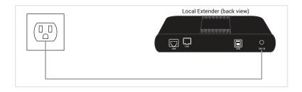
Power the Local Extender with the included 24-V, 1-A AC adapter and tighten the locking ring.
