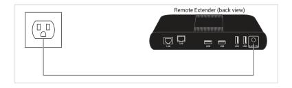
Power the Remote Extender with the included 24-V, 2.71-A AC adapter and tighten the locking ring.
