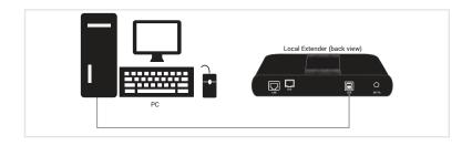
Connect the Local Extender to the computer's USB 3 port using the included USB cable.
