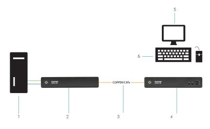
FIGURE 2-1. EMERALD EXAMPLE - UNMANAGED BASIC INSTALLATION
