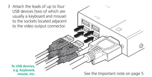
[MS2 variant only] Note: When connecting four USB devices to the unit, ensure that their total power requirements do not exceed 1700mA (1.7A). The USB standard states a maximum allowable current draw of 500mA (0.5A) per device, although most devices remain well below this limit - USB keyboards and mice typically require 100mA. Each X50 contains a self-resetting fuse that will prevent damage by shutting down the unit if the total power draw becomes excessive.
