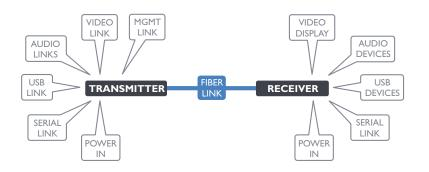
Note: In order to maintain a high level of confidence in the fiber optic link, the SFP's used must be those supplied by Adder: (SFP-MM-LC-4G or SFP-SM-LC-4G).
