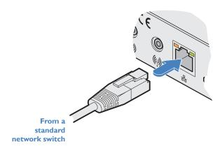
By default, the IP address is set to 192.168.1.22. If required, you can change the default IP address or alternatively, choose automated address selection by DHCP server. For details, please see the Configuration section.
