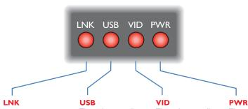
This indicator will be on once the link between the transmitter and receiver modules is established.
