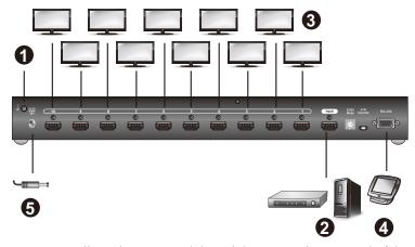
1. Use a grounding wire to ground the unit by connecting one end of the wire to the grounding terminal, and the other to a suitable grounded object.
