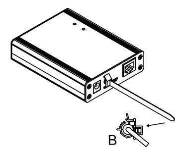
4. Connect the power adapter through the DC Jack Lock component B's joint as pictured below.
