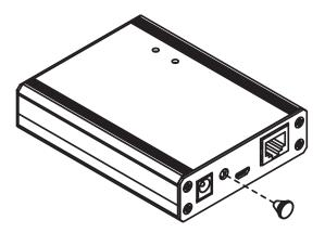
2. Insert the DC Jack Lock component A into the hole as pictured below.
