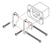
Figure 2.1 Retention Bracket assembly
