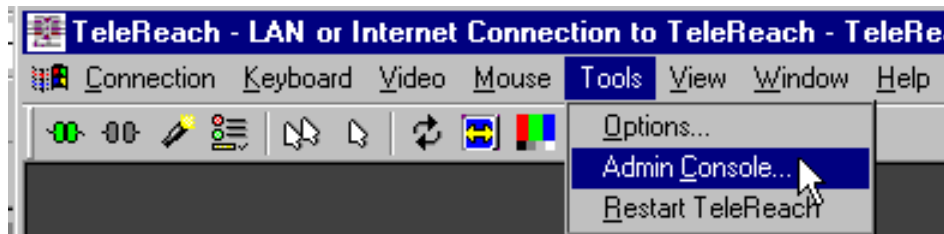
Figure 67. Accessing Admin Console Window
