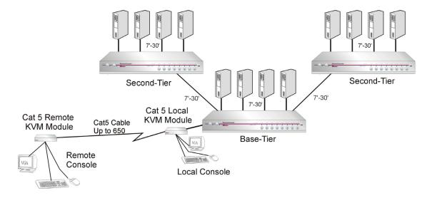
Figure 2. Two-Tier Configuration (With optional Remote Access)
