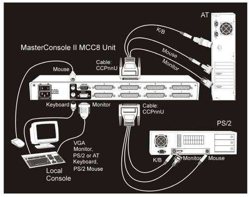
Figure 4. One-Tier Configuration Cabling Details
