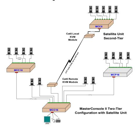
Figure 28. Two-Tier Configuration with Satellite Unit
