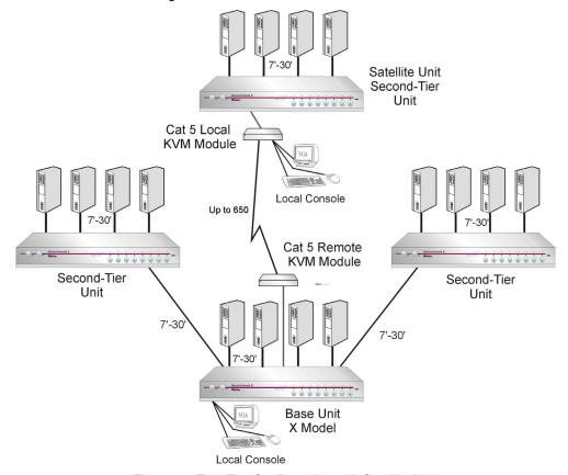
Figure 23. Two-Tier Configuration with Satellite Unit
