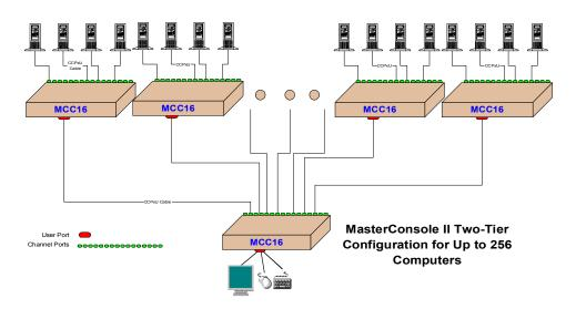
Figure 26. Two-Tier Configuration of up to 256 Computers
