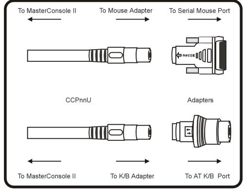
Figure 5. Cable Adapters to convert PS/2 to AT
