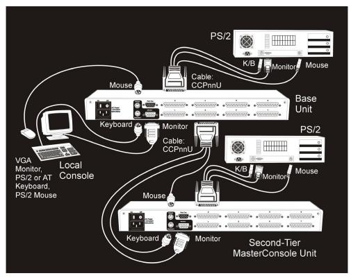
Figure 13. Two-Tier Configuration Cabling Details
