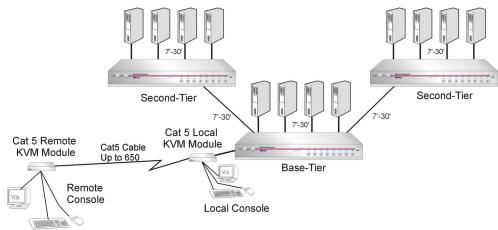
Figure 12. Two-Tier Configuration (With optional Remote Access Kit)
