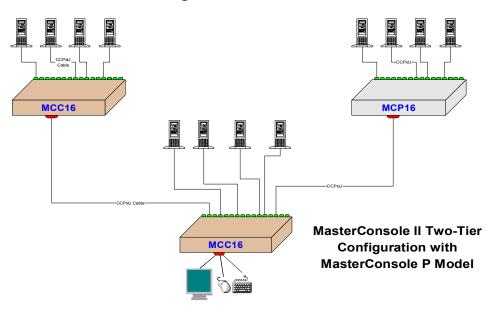
Figure 27. Two-Tier Configuration with MasterConsole P Model
