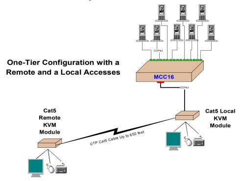
Figure 25. One-Tier with Remote Access Kit
