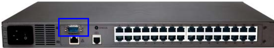
Figure 71 Factory Reset Connector Location
