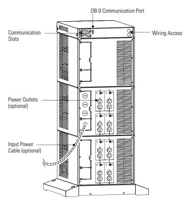
Figure 4. Nine-Slot Cabinet (Rear View)
