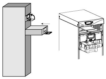
Figure 49. Inserting the Modules
