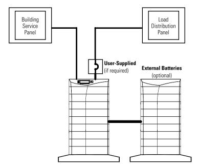
Figure 26. Typical Installation without a Bypass Switch
