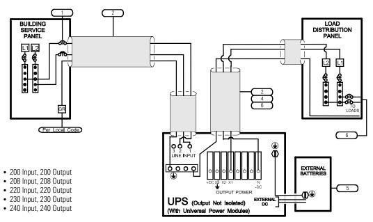
Figure 34. No External Bypass (L1, L2), Non-Isolated Output, and Universal Power Modules
