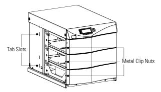
Figure 9. Metal Clip Nut and Tab Slot Locations
