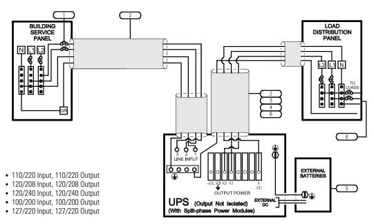
Figure 33. No External Bypass (L1, L2, N), Non-Isolated Output, and Split-Phase Power Modules
