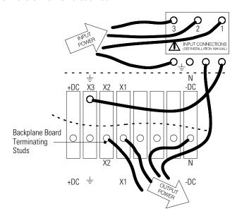
Figure 16. UPS Input and Output Terminals
