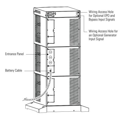
Figure 15. UPS Power Entrance Panel (Nine-Slot Cabinet Shown)
