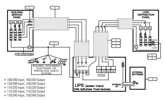
Figure 40. No External Bypass (L1, L2, N), Isolated Output for Single-Phase Voltages
