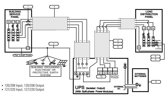
Figure 42. No External Bypass (L1, L2, N), Isolated Output for Derived Three-Phase Voltages
