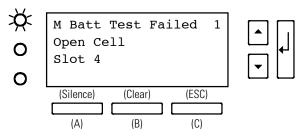
Figure 63. Detailed Alarm Entry
