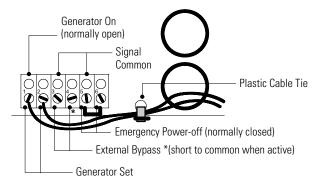
Figure 22. Input Control Signal Wiring (for External Controls)
