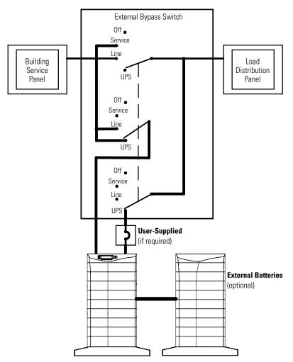
Figure 13. Typical Installation with a Bypass Switch
