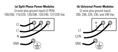
Figure 18. UPS Input Wiring
