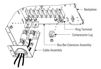
Figure 45. Bus-Bar Extension Installation
