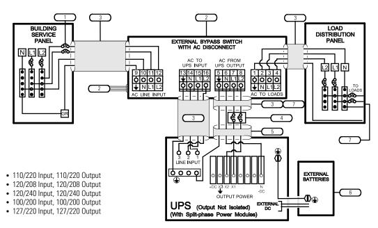
Figure 23. External Bypass Switch (L1, L2, N), Non-Isolated Output, Split-Phase Power Modules
