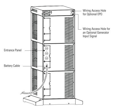
Figure 27. UPS Power Entrance Panel (Nine-Slot Cabinet Shown)
