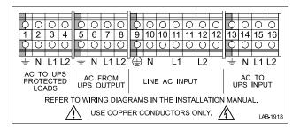
Figure 17. Bypass Switch Wiring Label
