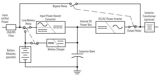
Figure 54. Powerware 9170+ UPS Functional Block Diagram
