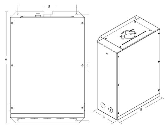
Figure 14. Bypass Switch Dimensions
