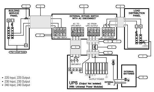
Figure 25. External Bypass Switch (L1, N), Non-Isolated Output, Universal Power Modules
