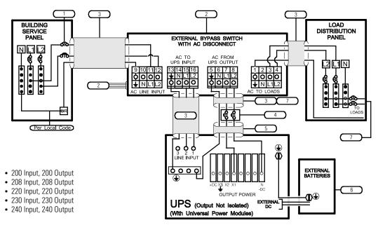
Figure 24. External Bypass Switch (L1, L2), Non-Isolated Output, Universal Power Modules
