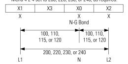
Figure 36. Isolated Outputs – Single-Phase Voltages
