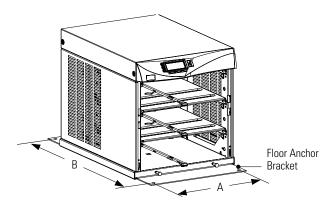
Figure 12. Floor Anchor Brackets Bolted to UPS Cabinet
