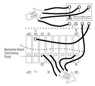
Figure 28. UPS Input and Output Terminals
