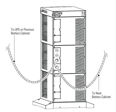
**Figure 48. Connecting Additional Battery Cabinets**
