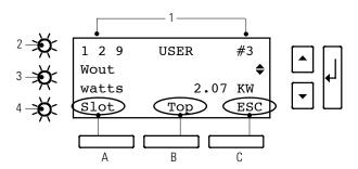
Figure 55. UPS Front Panel
