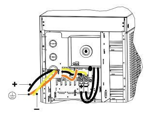
Figure 47. Battery Cable Installed in Battery Cabinet
