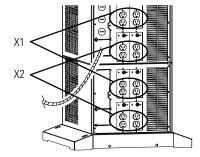
Figure 51. Balancing Receptacle Loads
