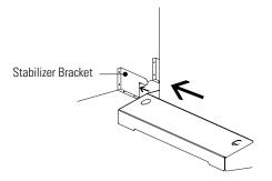
Figure 8. Stabilizer Bracket Installation
