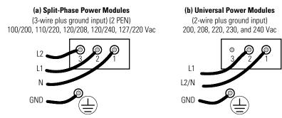
Figure 29. UPS Input Wiring
