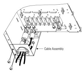
Figure 46. Battery Cable Assembly Installation
