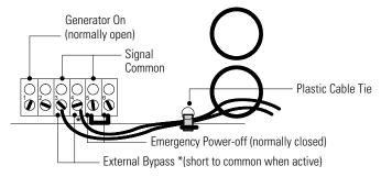
Figure 21. Input Control Signal Wiring (for MBB Bypass Switch)
