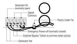
Figure 32. Input Control Signal Wiring
