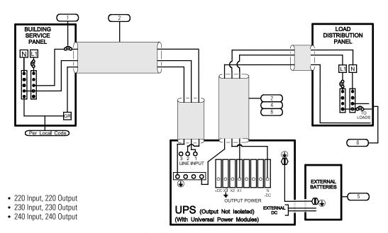
Figure 35. No External Bypass (L1, N), Non-Isolated Output, and Universal Power Modules
