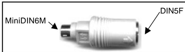
Figure 3-11: The AT Keyboard Adapter
