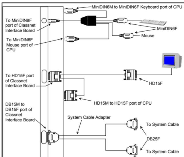
**Figure 6-4 Student PS/2 Cable Diagram**
