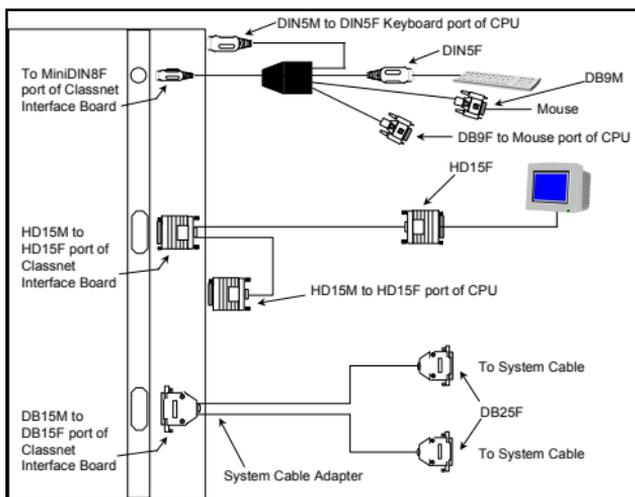
**Figure 6-3 Student AT Cable Diagram**
