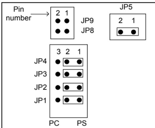
**Figure 5-3 Jumper Settings for PS/2**
