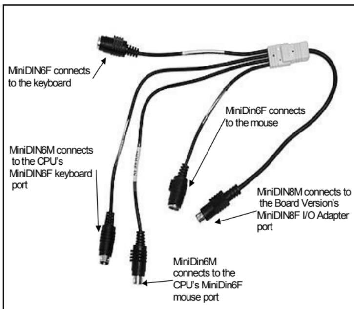
**Figure 6-12 I/O Adapter Cable for PS/2 - 5CB10041**
