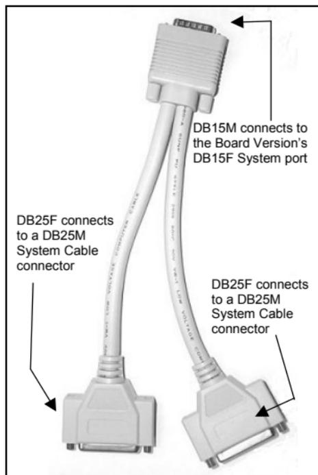
**Figure 6-6 The Student System Cable Adapter - 5CB10044**
