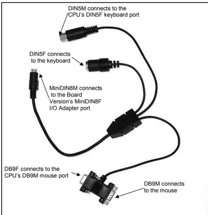
**Figure 6-11 I/O Adapter Cable for AT - 5CB10042**
