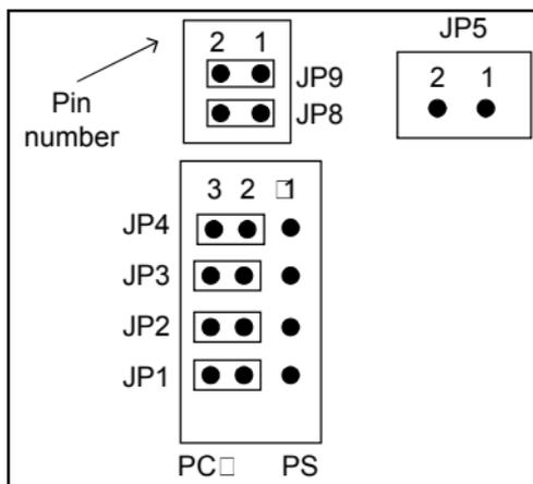
**Figure 5-2 Jumper Settings for AT**
