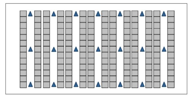
As with temperature sensors, humidity sensors should always be mounted consistently throughout the data center.
