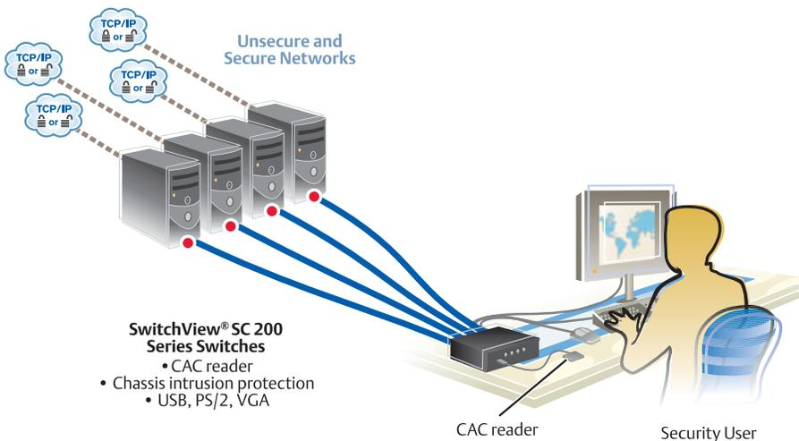
CAC support allows desktop IT administrators to deploy a single CAC reader that can be switched to all computers connected to the switch.
