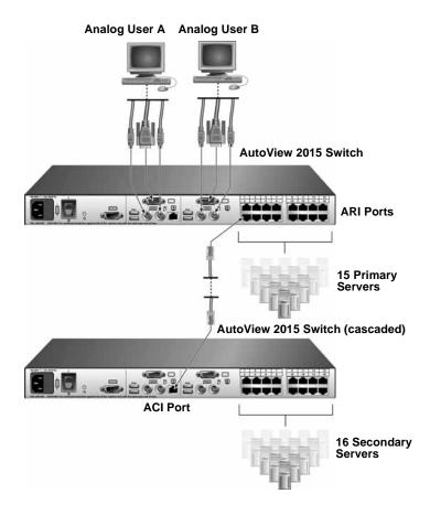
Figure 2.3: AutoView 2015 Switch Configuration with a Cascaded Switch
