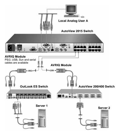
Figure 2.4: AutoView 2015 Switch Configuration with Legacy KVM Switches
