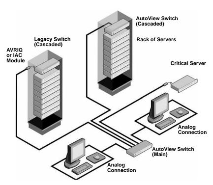
Figure 1.1: Example of an AutoView Switch Configuration
