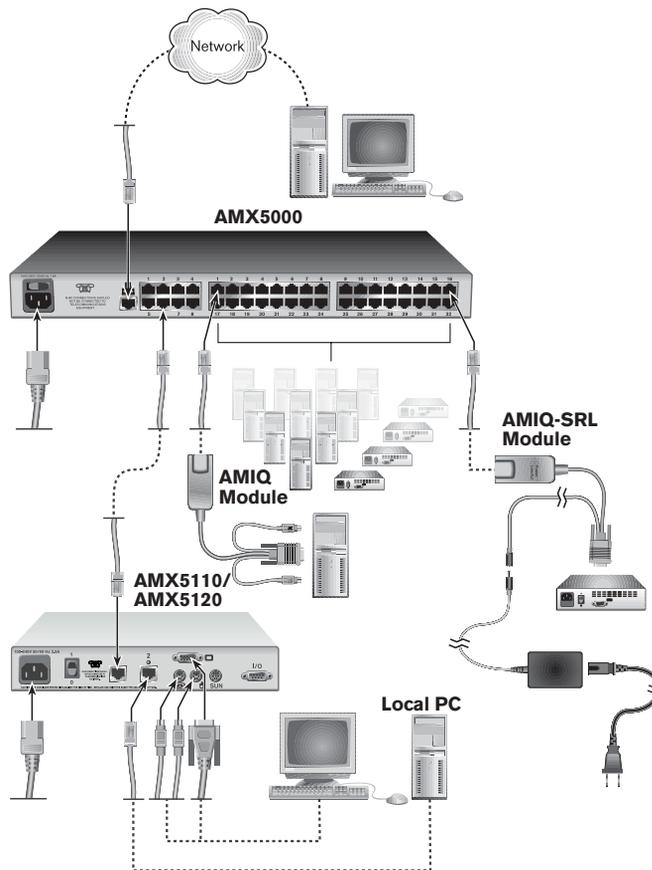
**Figure 2.1: Basic AMX Configuration**
