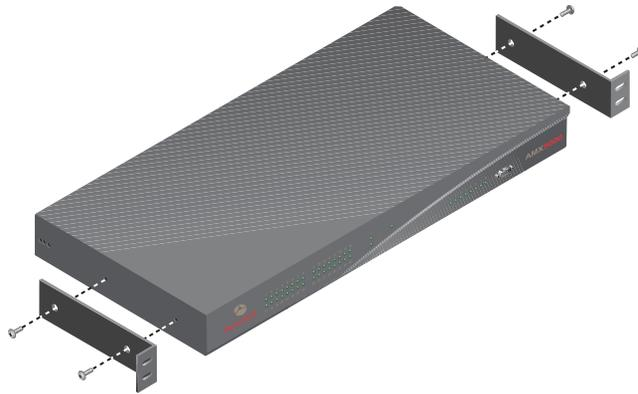
**Figure 2.4: AMX5000 Rack Mounting Diagram**
