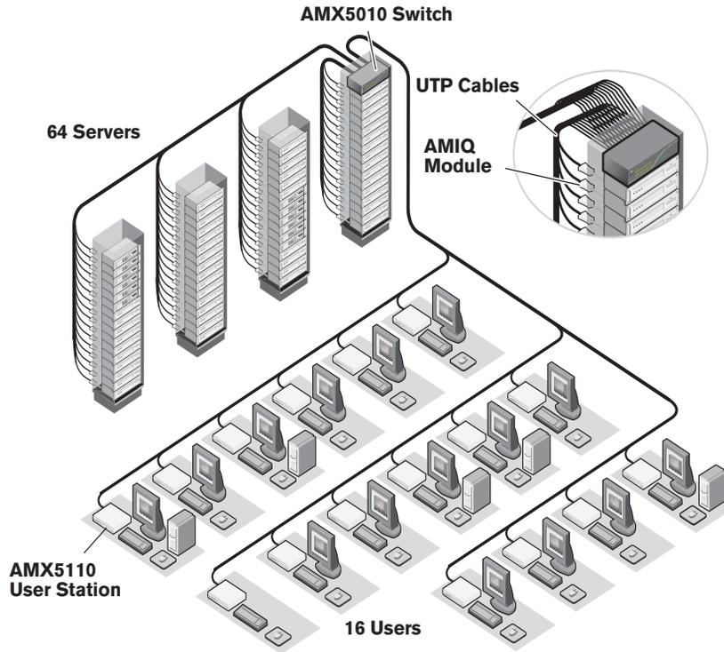
**Figure 1.2: Typical AMX Configuration**
