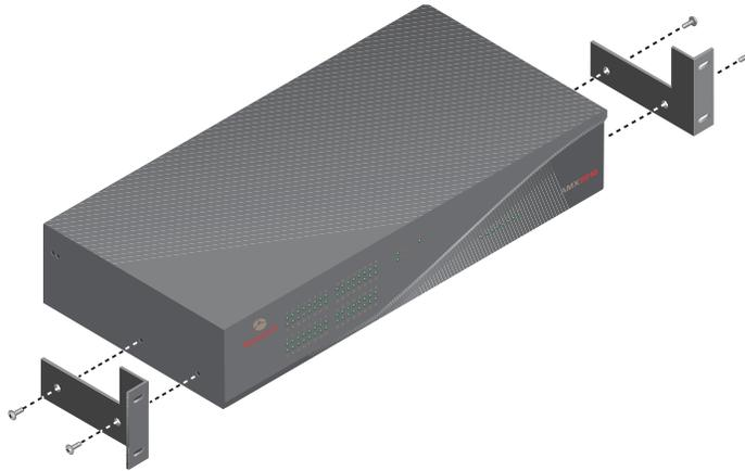
**Figure 2.5: AMX5010 Rack Mounting Diagram**
