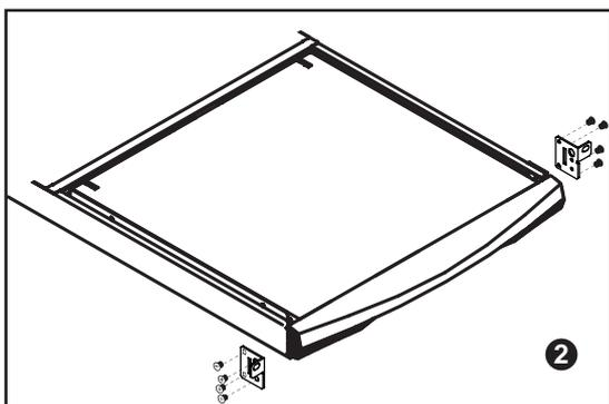
■ Install the optional front mounting ears with M3.2\*4.5mm screw x 8 pcs.
