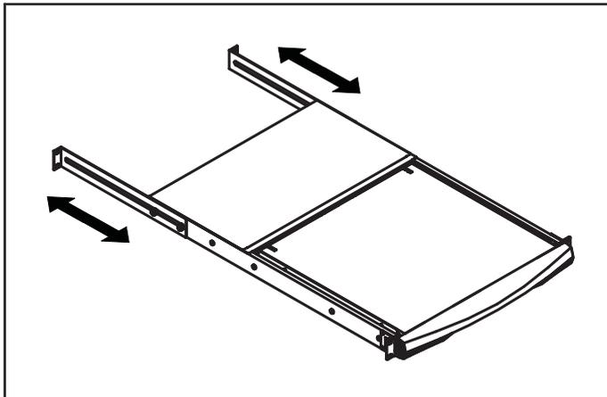
Figure 2. Aligning the rear L-brackets to a suitable length for the rack.
