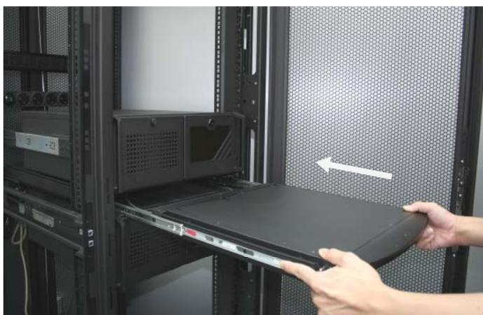
Figure 9. Pushing the LCD keyboard drawer into the rack.
