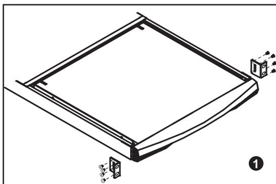
■ Disassemble the standard front mounting ears carefully.
