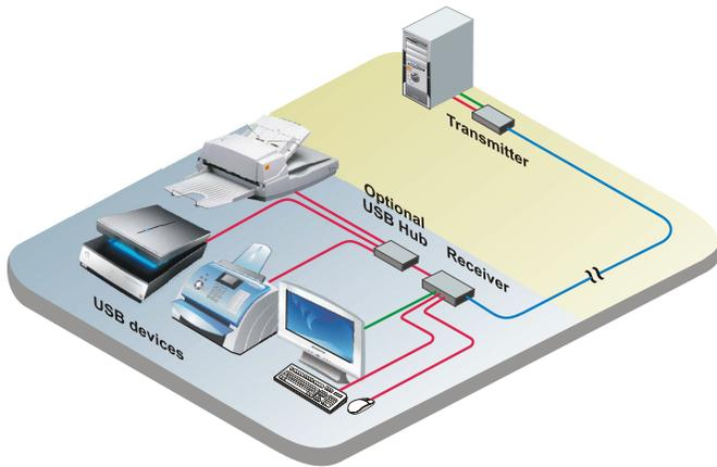
**Introduction** The CrystalView EX DVI extender consists of a local Transmitter unit and a remote Receiver unit connected by up to 330 feet (100 meters) of CATx cable. The Transmitter unit connects to a computer's DVI video, and USB port. The Receiver unit connects to the console DVI display and USB 1.1 or 2.0 devices.
