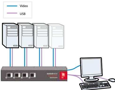
The switching section is hardwired to allow only one channel to be selected at any time.
