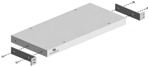
Figure 2.1: AutoView Switch Horizontal Installation
